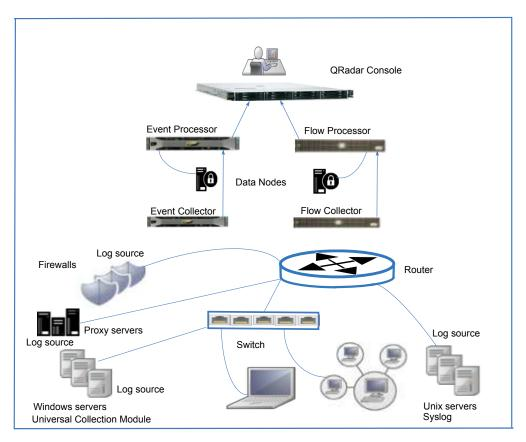
Figure 4. QRadar event and flow components
