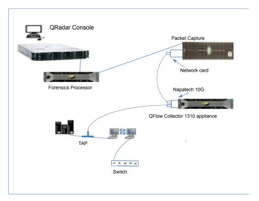
Figure 15. Packet data forwarding from a QRadar QFlow Collector to QRadar Packet Capture by using the Napatech card
