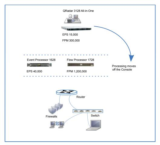
Figure 7. Adding processing capacity
